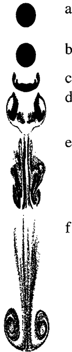
FIG. 19. Cross section of the blob at different non-dimensional times ( tU/D ) (Case 3). (a) 0.03, (b) 0.75, (c) 1.47, (d) 2.91, (e) 7.21, and (f) 21.57.
